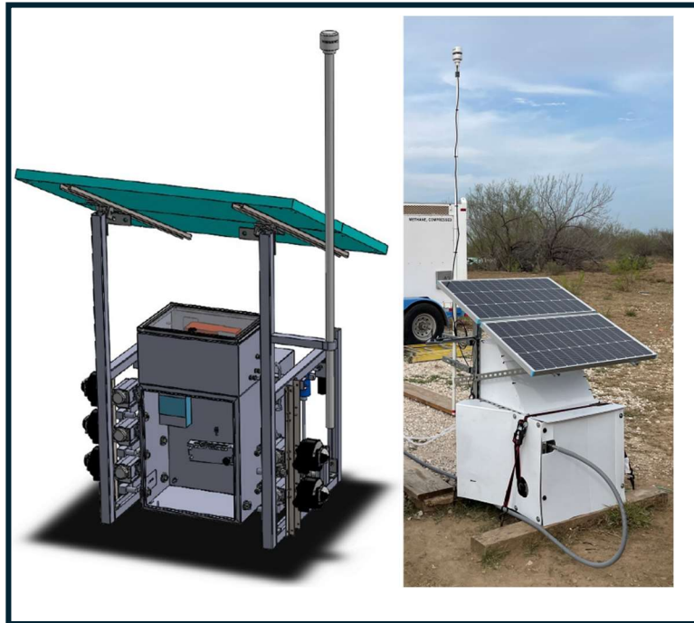
Figure 1: (Left) conceptual CAD model; (Right) Controlled Release Rig as built, in use during testing.
