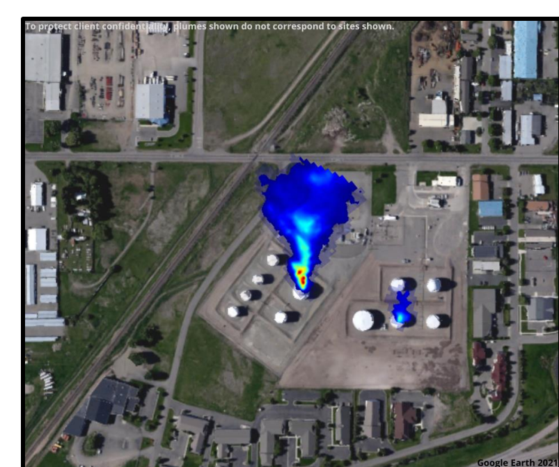
Figure 3: (Generic) Example of methane plume image captured by aerial instrument
